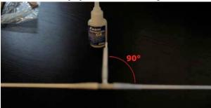
3. Glue the bottom fuselage half to the bottom of the wing. Again, make sure that it is perpendicular to the wing surface.
