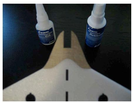
2. Glue the top fuselage half onto the top of the wing using foam-safe CA. The tabs will align the fuselage horizontally, but make sure that it is mounted perpendicular to the wing.
