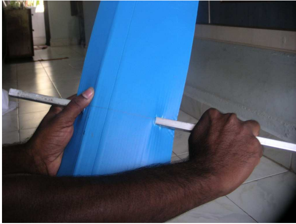
➤ Insert Fuse tube into wing
