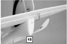
14. Slide the elevator in its slot, so it fts properly to the fuselage. Control there is no gap and the cam fts in the slot of the fuselage.
