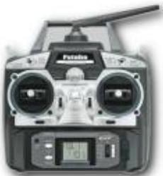
The first problem with the Futaba FASST systems was the zero GUID issue which saw some sets losing a small but critical part of their memory which resulted in multiple systems interacting in a rather unpleasant way. In effect, two systems that suffered this problem could end up shooting each other down.
