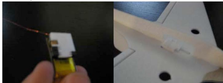
5. If you would like to add a decorative finish to your Komet, do so now before mounting the electronics. You can use foam-compatible spray paint, markers, or printed tissue. This model was airbrushed using thinned Testors Gloss Red Enamel.
