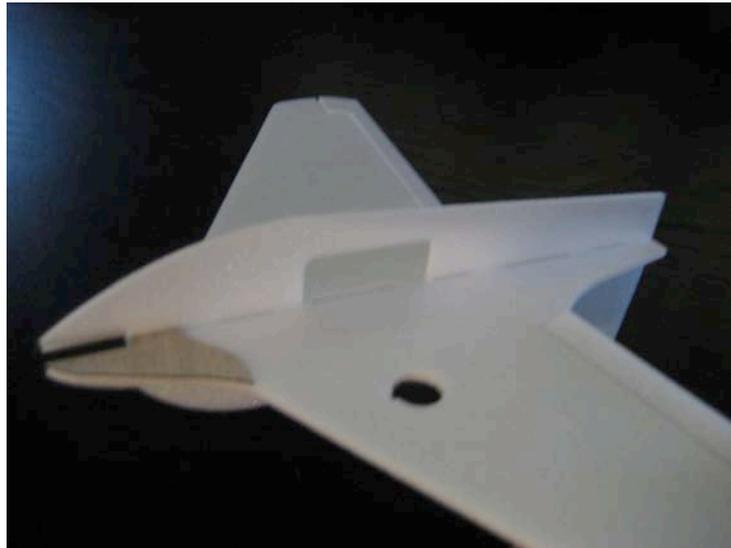
4. Press the foam receiver mount onto the HFX900 receiver and attach an LP90 cell. Move the assembly around until it is centered inside the receiver cutout on the fuselage, then mark its position. Glue the foam mount in place, then remove the receiver and battery.
